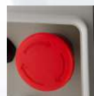
Emergency stop Interruptor emergencia
